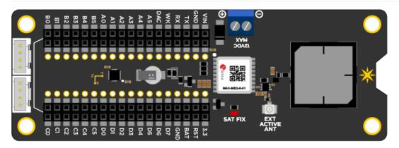
This new revision of the Electron Asset Tracker uses a uBlox M8 engine GNSS receiver. Unlike the v1, this module is capable of receiving 3 GNSS (GPS, Galileo, GLONASS, BeiDou) concurrently. We have also added a low noise amplifier and a band pass filter for improved performance with the on-board antenna.
